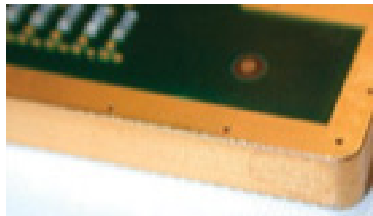
Via Fencing and Edge Plating for EMI Suppression
