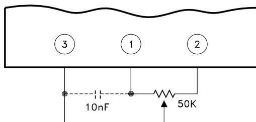
Adjust/comp (pin 3) may be driven by external circuitry referenced to pin 2 (-output) if desired. Grounding pin 3 causes voltage to increase (25% typically) while driving pin 3 above 1.3V causes output voltage to decrease. Pin 3 may be driven through 10KΩ or more if connection of the comp function is also required.
