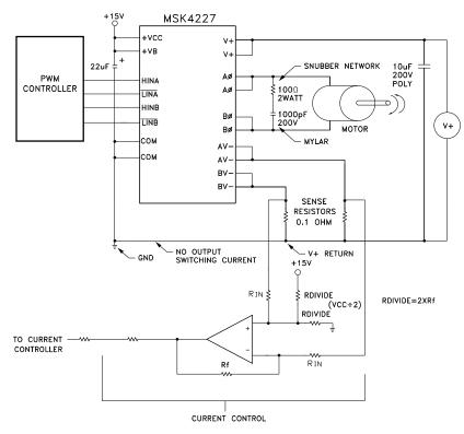
This is a diagram of a typical application of the MSK4227. The design +VCC voltage is +15 volts and should have a good low ESR bypass capacitor such as a tantalum electrolytic. The digital inputs can come from a microprocessor or any type of PWM controller. The controller will use the current sense signal to either control current through PWM, current limit the bridge, or both.
