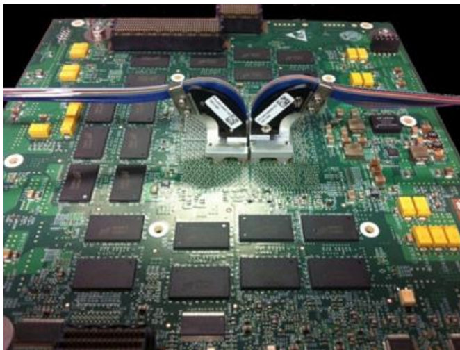
Fig. 3. PCB with assembled optical interconnect and fiber bundles.
