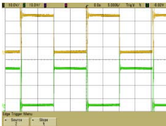
Bridge outputs at zero amps. 50% duty cycle.
