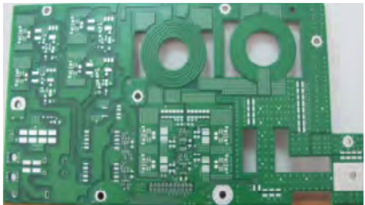
4-Layer, 6 oz PCB: TTM Zhongshan (ZS) is dedicated to the Automotive industry. This is an example of a heavy copper board produced at that site.
