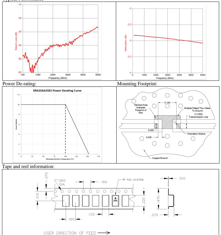
TAPE DETAIL & RF PAD ORIENTATION
