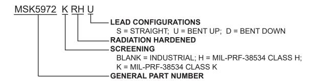
The above example is an adjustable Class K regulator with leads bent up.
