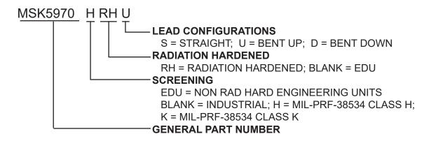
The above example is an adjustable Class K regulator with leads bent up. Ordering information for the 3 pad ceramic SMD-1 package is contained on the next page.
