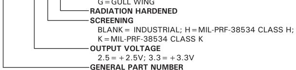
The above example is a +2.5V, Class K regulator with gull wing formed leads. NOTE: See DSCC SMD 5962F09209 for DSCC part number options.
