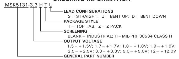
The above example is a +3.3V, Military regulator using the top tab package with leads bent up.
