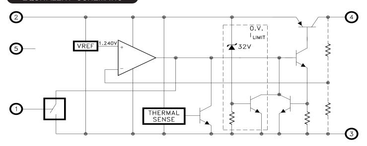
Schematic shown for fixed output voltage versions
