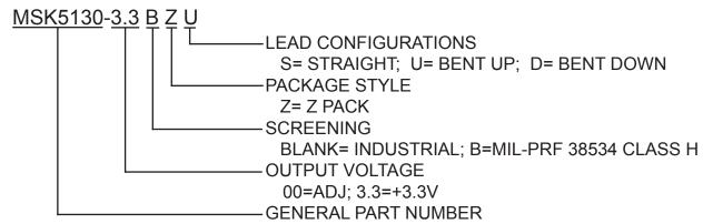
The above example is a +3.3V, Military regulator using the top tab package with leads bent up.
