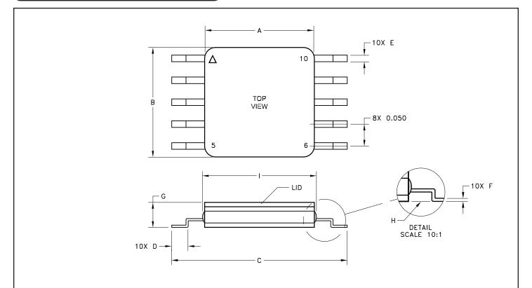
NOTE: LEADS SHALL BE COPLANAR (H) WITH THE PACKAGE BASE.
