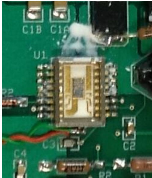
Fig. 5: Photography of the die with the melting thermal compound under it (in white color)
