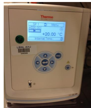
Fig. 4: Photography of the Cooling Plate Controller (Temperature is set at 20°C)
